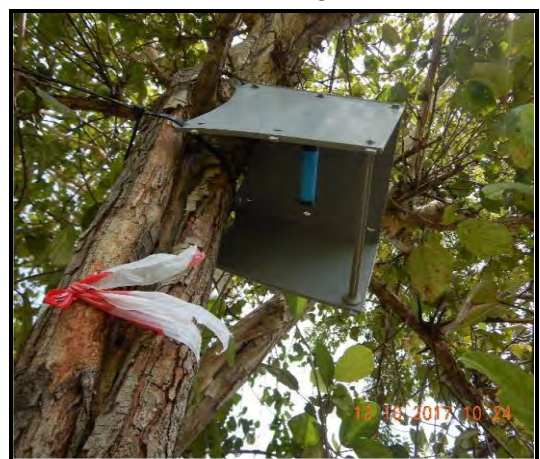
Plate 8: NO 2 & SO 2 measurement at Awura Forest
