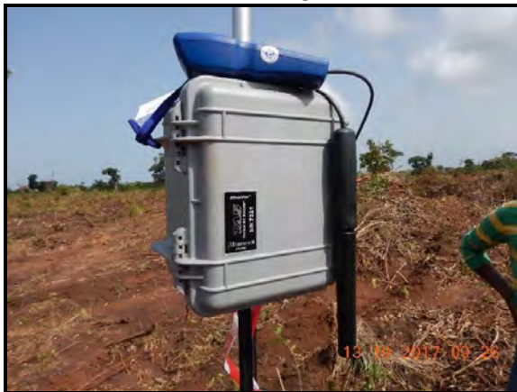
Plate 3: TSP & PM10 monitoring at Chirimfa Forest
