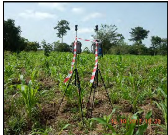
Plate 4: Noise measurement at Chirimfa Forest
